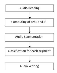
Figure C2.1. Audio segmentation stages.
