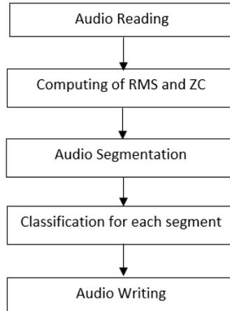
**Figure C1.1.** Audio segmentation stages.
